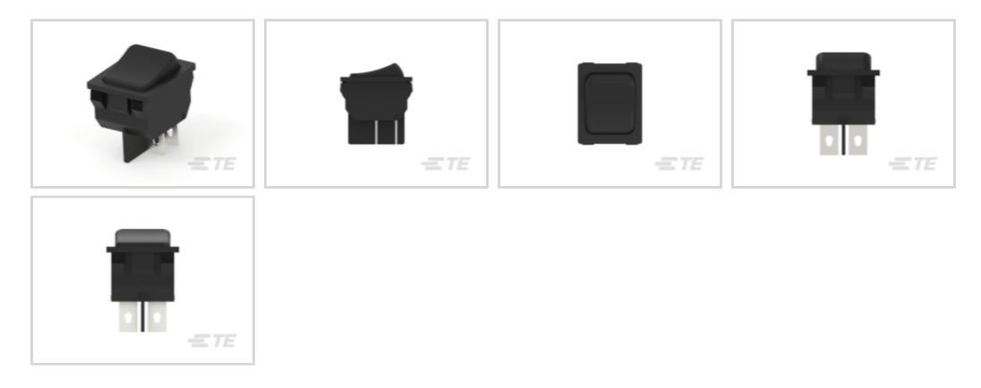
Rocker Switch Type: Power Rocker Switch Mounting Type: Panel Indicator/Imprint Legend: None Panel Cutout Size: 30.2 x 22.2 mm [ 1.19 x .874 in ] Switch Contact Plating Material: Silver Tin Oxide
